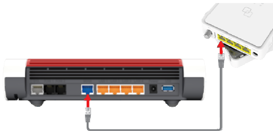
Fig. 1: Connect FRITZ!Box to the ONT using a LAN cable
